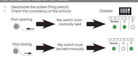
In case of inconsistency between actions, check the wiring of the installation.
