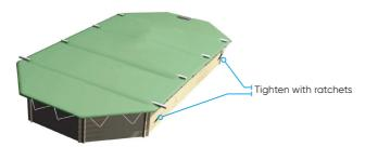
Tension the cables in the cover bars.
