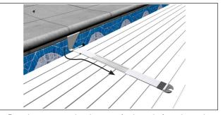
• Run the strap under the straplock and place it on the slatted cover
