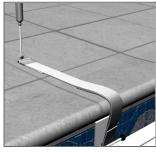
Run the strap between the wall and the straplock rod
