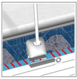
The slatted cover must not exit the Quicklock before the key switch has been pressed.
