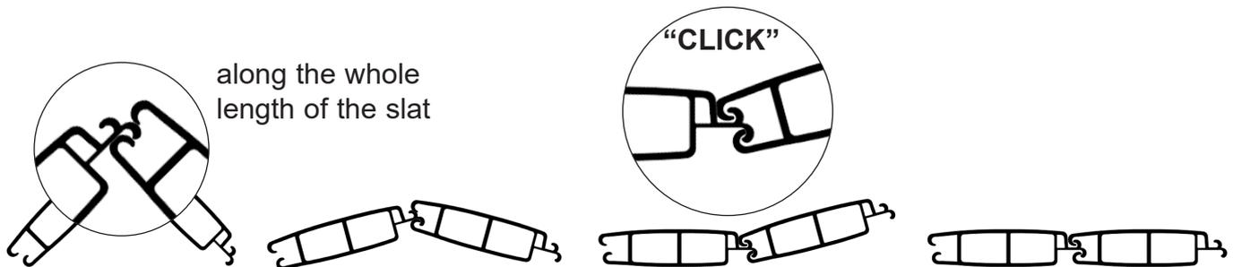
Repeat the movement until all the slats are completely clipped together
