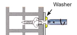
After reaching the resistance point, make 3 more turns of the screwdriver to finish tightening.
