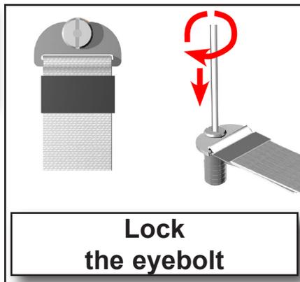
The strap must be tight and the cover must touch the bottom of the straplock
