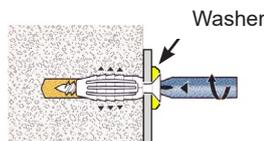
Once the resistance point has been reached stop screwing, this would deteriorate the fixture quality.
