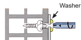
After reaching the resistance point, make 3 more turns of the screwdriver to finish tightening.
