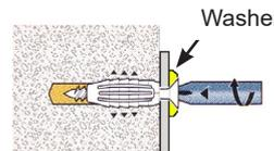
Once the resistance point has been reached stop screwing, this would deteriorate the fixture quality.
