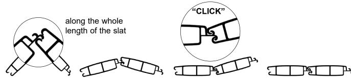
Repeat the movement until all the slats are completely clipped together
