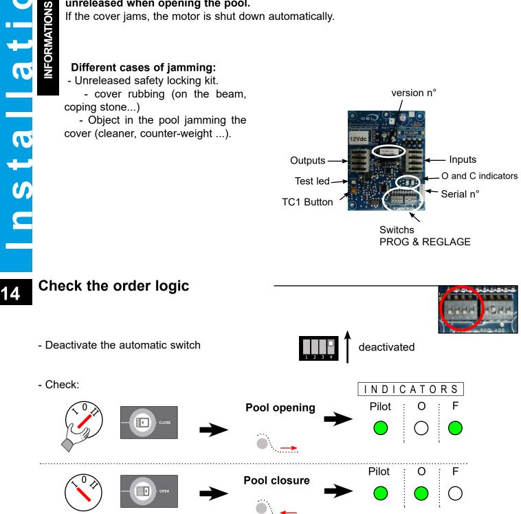
If the command logic is not correct, check the installation wiring.
