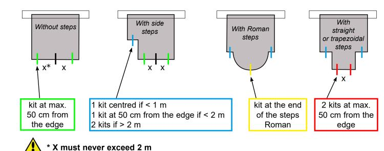
The Quick-lock fastener system cannot be used on cut off corners and curves, except at the end of Roman steps.
